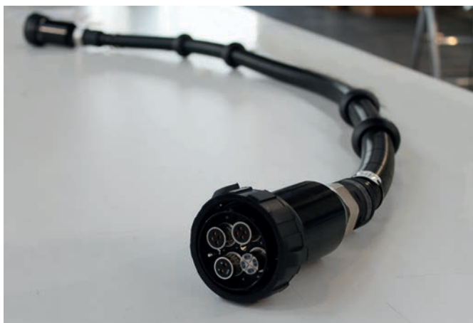
The finished harness - front view
