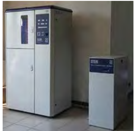
UV TEST MACHINE Q-SUN Xe-2 Xenon TEST CHAMBER
