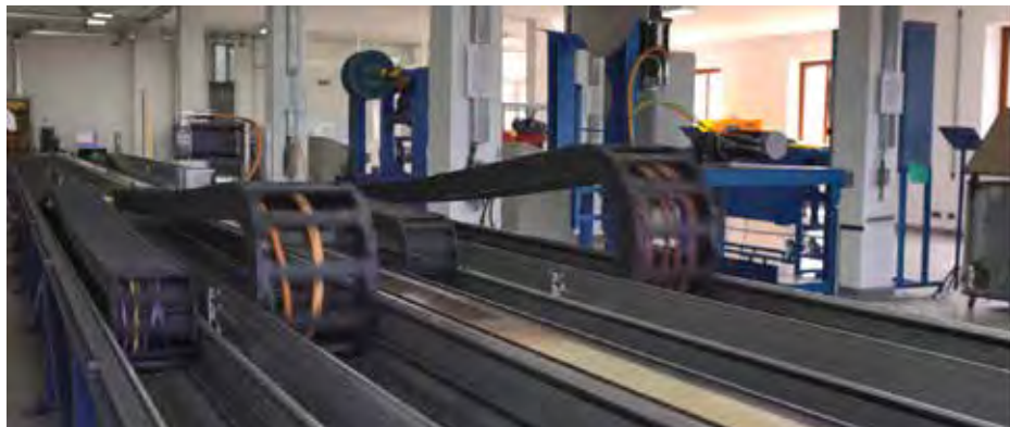
CHAIN WITH A LENGTH OF 18 m - TOP SPEED 200 m/min - MAXIMUM ACCELERATION 10 m/s 2
