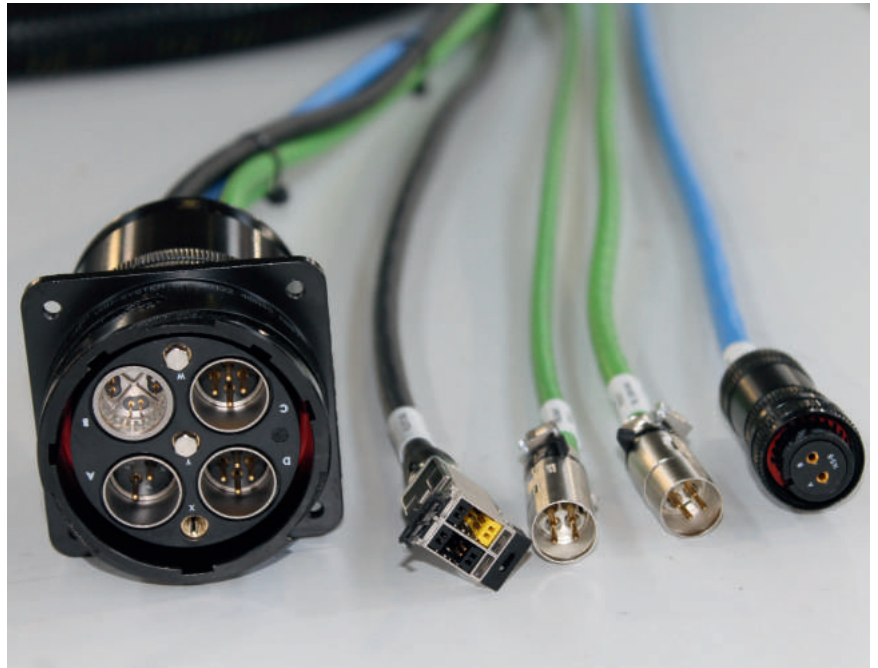
The finished harness - connectors detail
